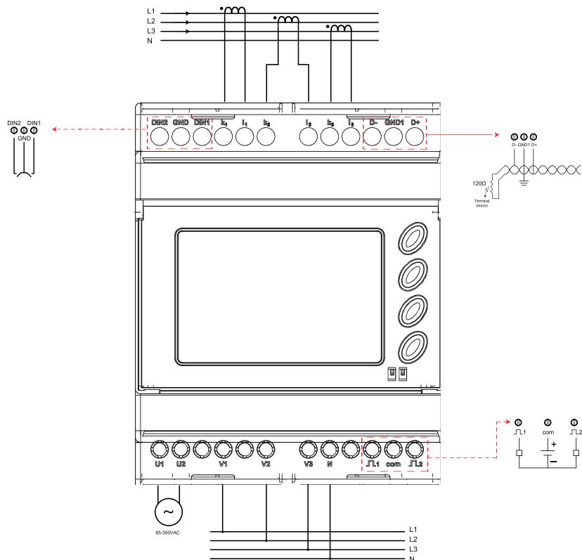
The connection diagram above is general for transformer connection devices and may vary depending on the model.
