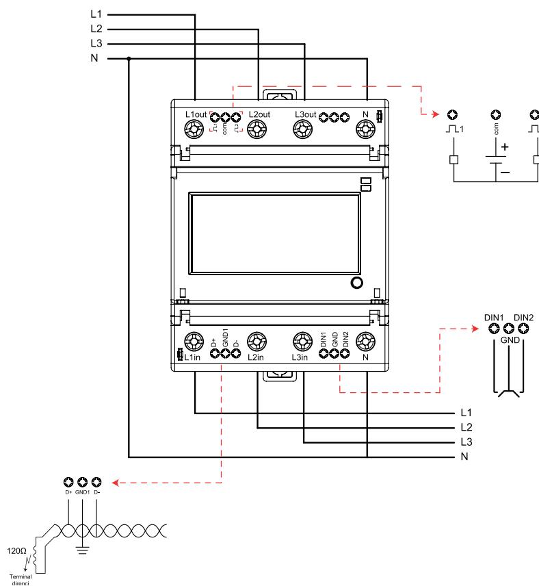
The connection diagram above is general for direct connection devices and may vary depending on the model.
