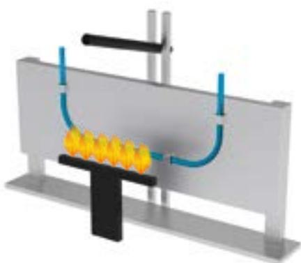
**IEC 61034-1/2 / EN 50268-1/2: Measurement of smoke density of cables burning under defined conditions.**
