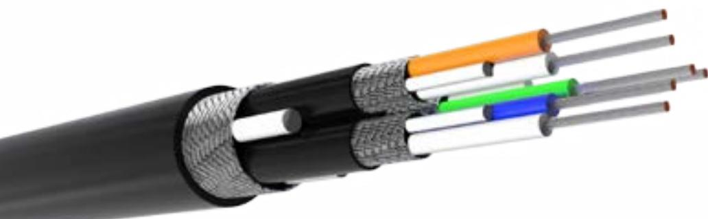
**MAIN FEATURES****TK-AUDIO 3x(2x0.60)****Conductor resistance** ≤ 37.0 Ω/km**Insulation resistance** ≥ 2500 MΩxkm**Test voltage** 2000 V**Characteristic Impedance @ 1 MHz** 110 ± 10 Ω**Mutual capacitance** ≤ 50 pF/m**Nominal Velocity of Propagation** 78%**Nominal weight** 335 kg/km**Nominal diameter** 15.5 mm
